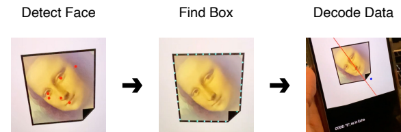
Figure 3: For each detected face, a CPU-based process checks whether it is surrounded by an external, solid-colored box. If a box is found, the relative orientation of the face to the box is evaluated to extract encoded information. Ninja Codes are detected/decoded in the exact same manner.
